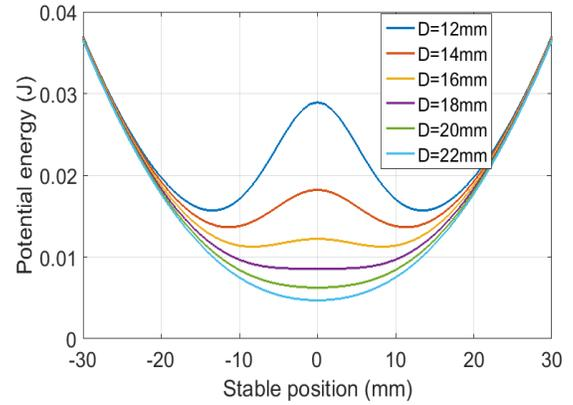
**Figure 3. The variation of the potential energy function as the distance between two magnets ( $D$ ) changes.**
