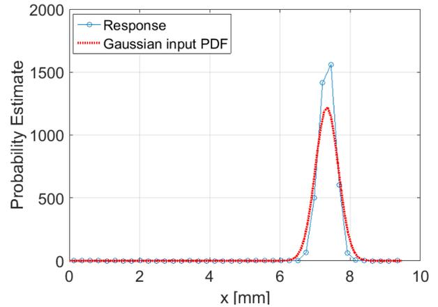
**Figure9. Probability density function of displacement for case III (D=15mm).**
