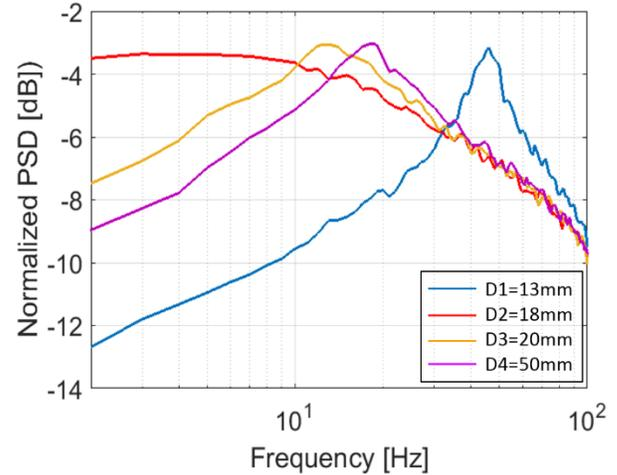
**Figure 12. Power spectral density of voltage as the distance between magnets varies when  $a_{rms} = 1g$ .**
