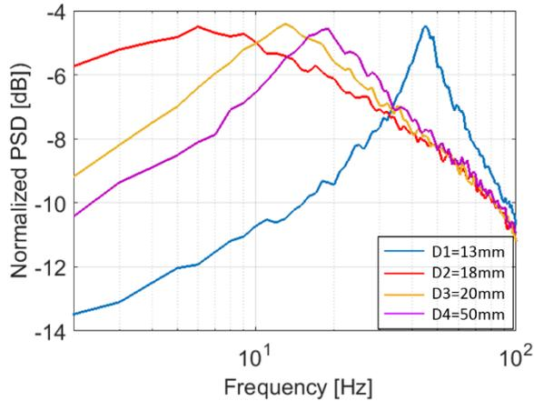
**Figure 11. Power spectral density of voltage as the distance between magnets ( $D$ ) varies when  $a_{rms} = 0.5g$ .**
