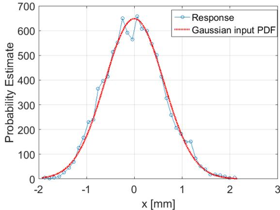
**Figure 7. Probability density function of displacement for case I (D=20mm).**
