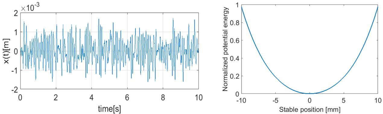
**Figure 4. Case I: when  $D=20\text{mm}$ , Left: displacement time response. Right: Potential energy function.**
