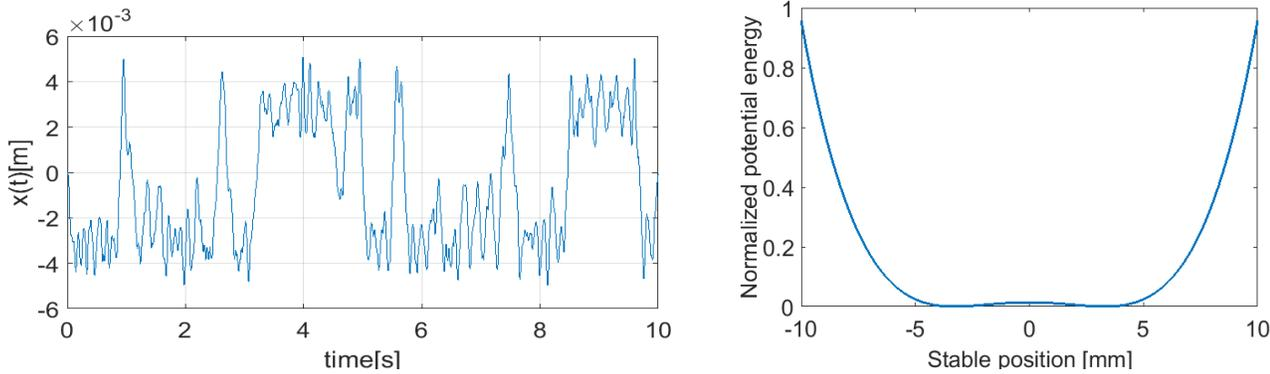
**Figure 5. Case II: when  $D=17.7\text{mm}$ , Left: displacement time response. Right: Potential energy function.**
