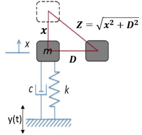
**Figure 2. Simplified model of the bi-stable resonator with two magnets.**
