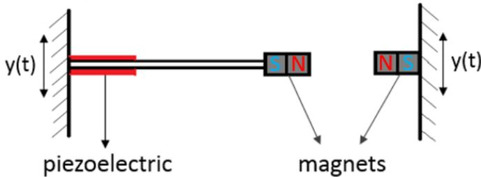
**Figure 1. A schematic diagram of the bi-stable resonator.**
