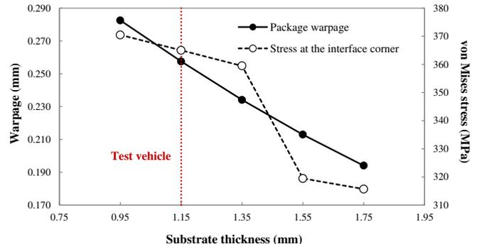
Fig. 16. Substrate thickness impact on package warpage and interface corner stress.
