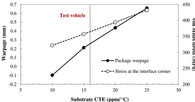
Fig. 14. Substrate CTE impact on package warpage and interface corner stress.
