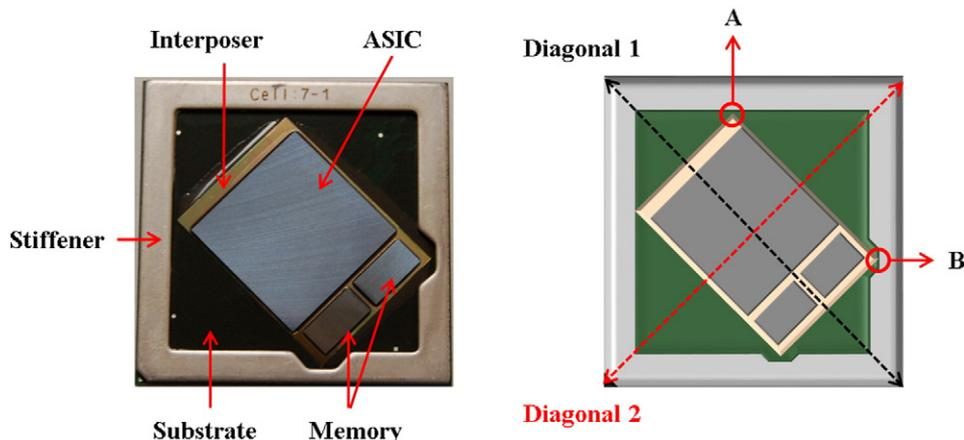
**Fig. 1.** Test vehicle (TSV interposer package).
