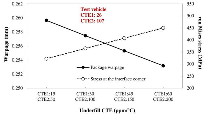
Fig. 11. Underfill CTE impact on package warpage and interface corner stress.
