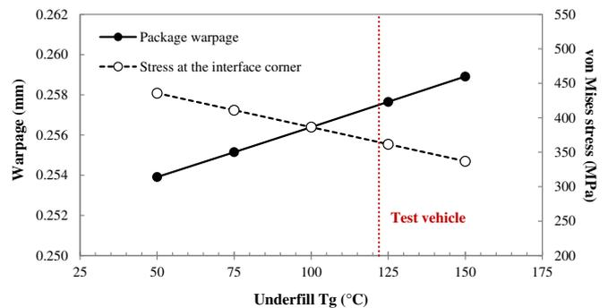
Fig. 12. Underfill  $T_g$  impact on package warpage and interface corner stress.
