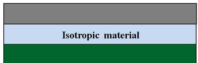
Fig. 6. Simplification of the composite layer by the effective material property.
