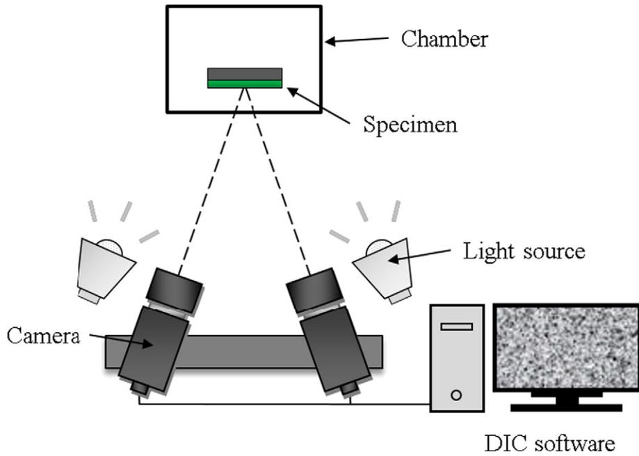
Fig. 3. Schematic of 3D DIC system setup.
