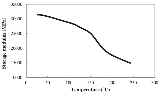
Fig. 5. Substrate modulus measurement result.
