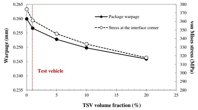
Fig. 15. TSV (Cu) volume fraction impact on package warpage and interface corner stress.
