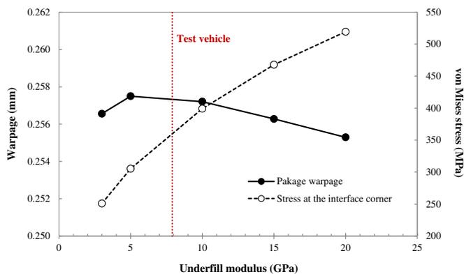
Fig. 10. Underfill modulus impact on package warpage and interface corner stress.
