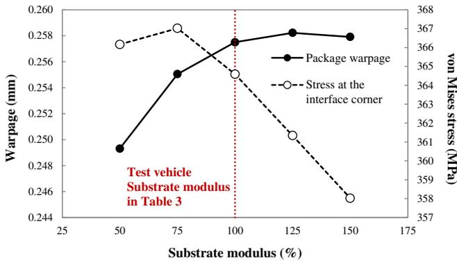
Fig. 13. Substrate modulus impact on package warpage and interface corner stress.
