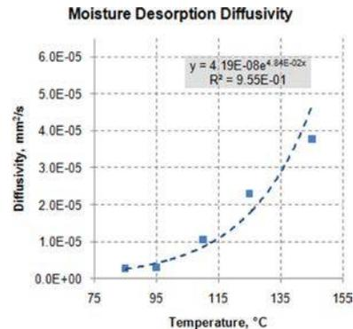
Figure 5 Moisture desorption properties following Arrhenius equation
