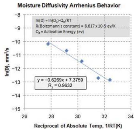
shows that the result follows Arrhenius equation, equation (5). From the result shown in Figure 3, the saturated moisture concentration appears to be influenced by temperature because the rate of volume change in mold compound is susceptible for temperature as previously mentioned. Based on the experimentally obtained  $C_{sat}$ ,  $C_{sat}$ 's for other temperatures can also be estimated by an extrapolation as shown in Figure 6.
