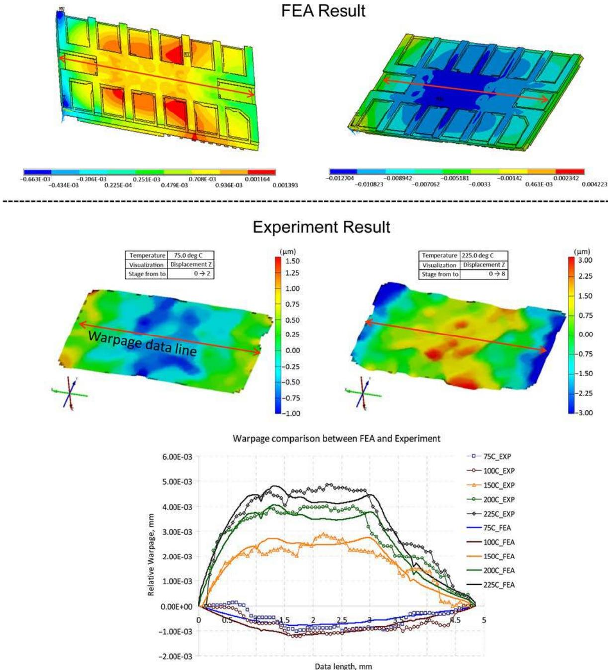
Notes: (a) Warpage contour plots at 75°C and 225°C; (b) Warpage line plot along middle section on BT core substrate side
