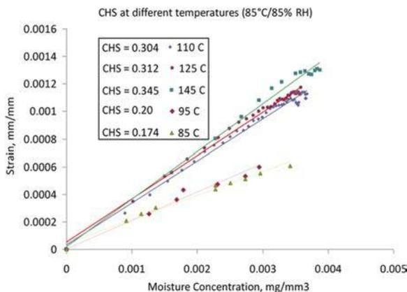
in the trend observed between 100°C and 120°C around the  $T_g$  (~110°C). Figure 10 shows that the experimental data agree with those by DIC quick scanning method. Also, the result shows CHS increases with respect to temperatures below and above  $T_g$ . These hygro-material properties are implemented in FEA simulation for further investigation of moisture effect on MEMS package.
