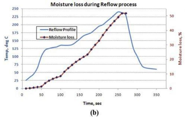
Notes: (a) Transient moisture contour; (b) average moisture loss during reflow
