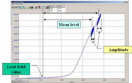
Fig. 5. Typical DMA testing profile.
