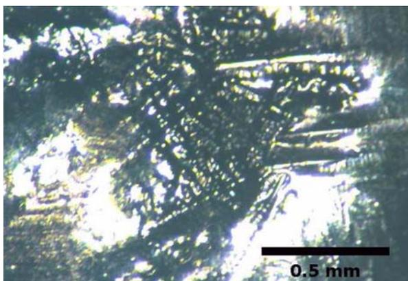
Fig. 8. A micrograph of indium solder with 4 nm of oxide after reflow in the inert environment.
