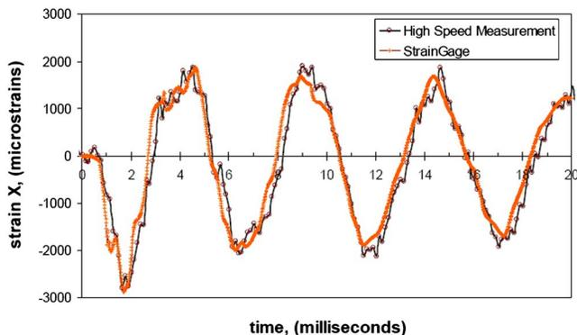
**Fig. 5 Test validation of high-speed DIC measurement compared with strain gauge for test board A**
