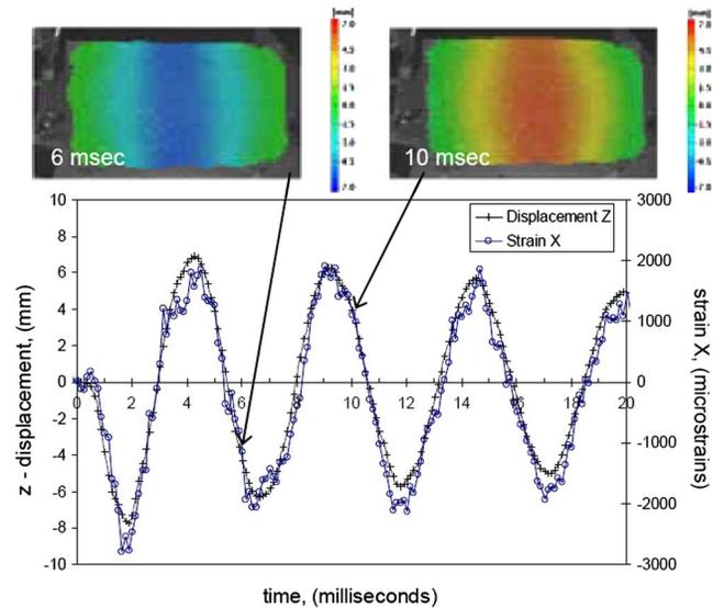
Fig. 3 Time-history of the out-of-plane displacement at the board center and in-plane strain at the strain gauge mounting location on test board A
