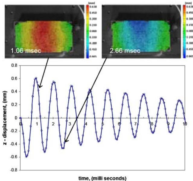
**Fig. 4 Time-history of the out-of-plane displacement at the center of test board B**
