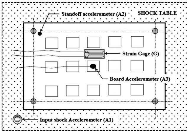
Fig. 1 The bottom of the board showing the position of the accelerometers and the strain gauge
