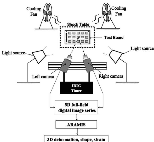
Fig. 2 Schematic of high speed measurement setup
