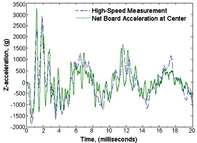
**Fig. 6 Test validation of high-speed measurement with accelerometer time history at the center of board A**
