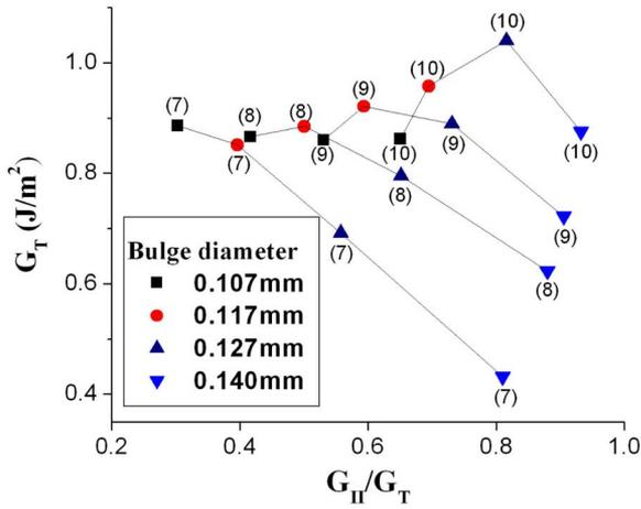
Fig. 13. Mixed-mode ratio versus strain energy release rate. (The number in parenthesis is pitch (unit: mil).)
