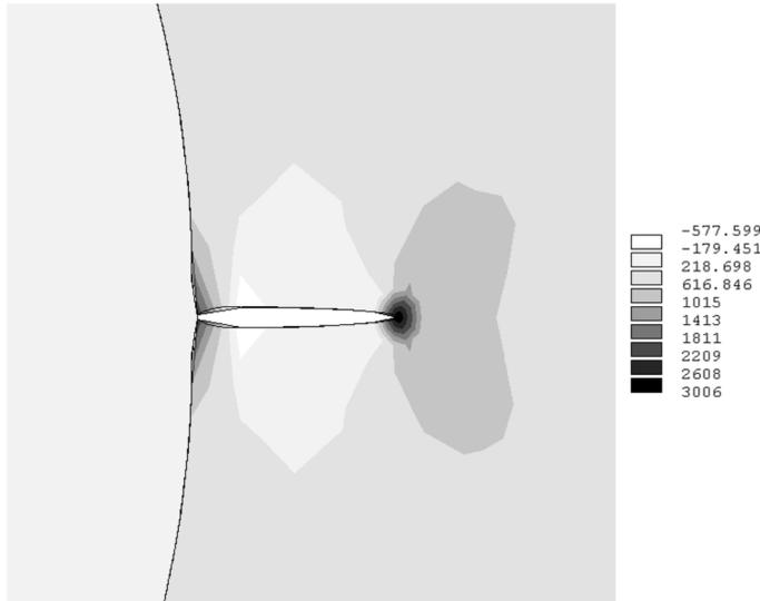
Fig. 14. Stress ( $\sigma_{yy}$ ) distribution around edge crack tip (case with edge crack).
