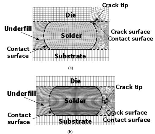
Fig. 2. Finite-element mesh of crack model.
