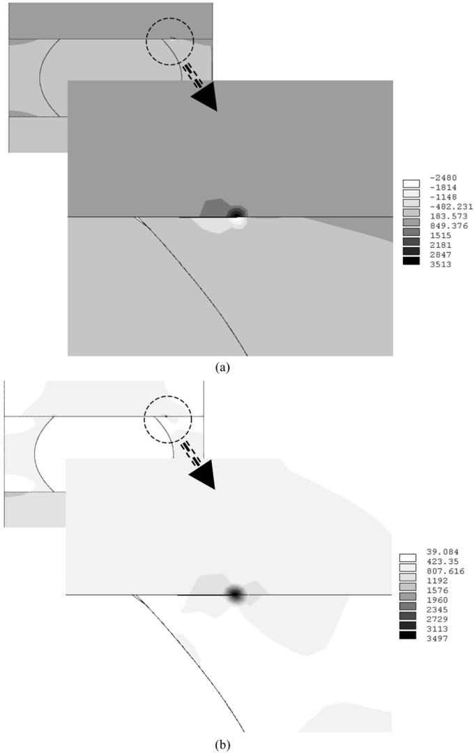
Fig. 7. Stress distributions in interfacial crack (right side of figures are the enlarged ones around crack tip).
