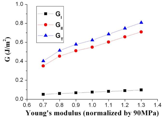
Fig. 10. Young's modulus of underfill versus strain energy release rate.
