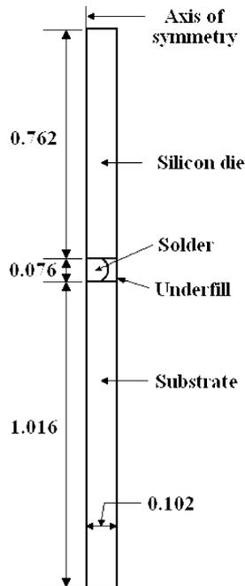
Fig. 1. Schematic of axisymmetric model used for analysis (unit: mm).
