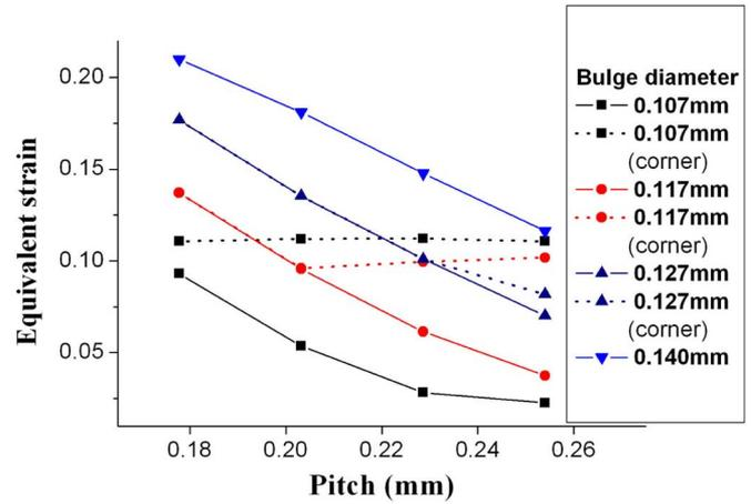
Fig. 16. Pitch versus maximum equivalent strain.
