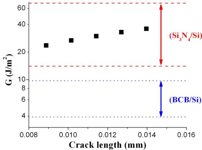
Fig. 11. Interfacial crack length versus strain energy release rate (at room temperature).
