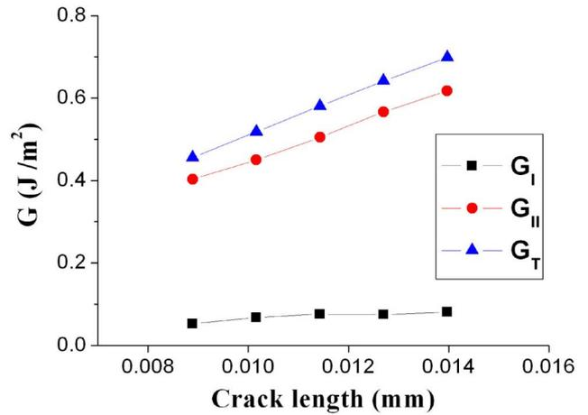
Fig. 9. Interfacial crack length versus strain energy release rate.
