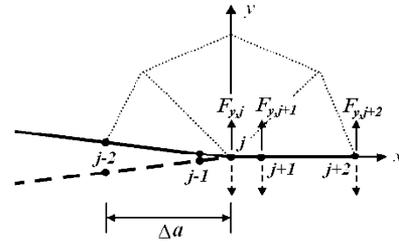
Fig. 8. Schematic mesh for modified crack closure integral.
