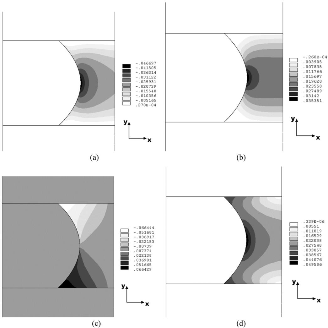
Fig. 3. Strain distributions (case without crack).
