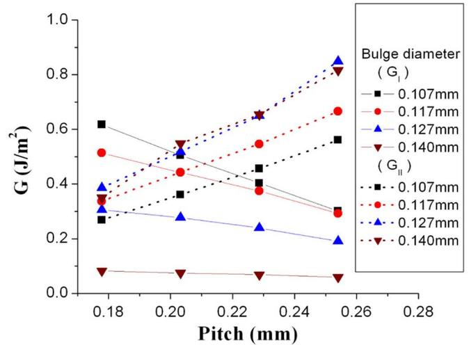
Fig. 12. Pitch versus strain energy release rate.
