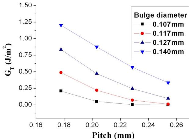
Fig. 17. Pitch versus total strain energy release rate.
