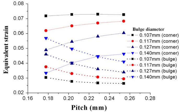
Fig. 6. Pitch versus maximum equivalent strain (at corner and bulge).
