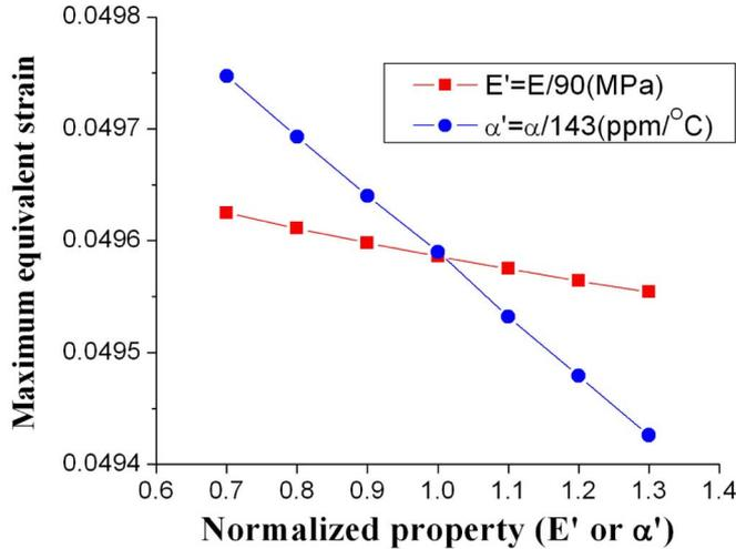
Fig. 4. Effects of underfill property (Young's modulus and CTE) on maximum equivalent strain.
