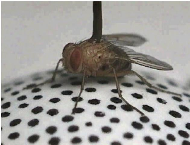
By using a free-floating ping-pong ball as a "fly treadmill," scientists were able to measure precise changes in the fly's direction of motion. Dots on the ball enabled tracking by computer. Copyright © Cornell University
