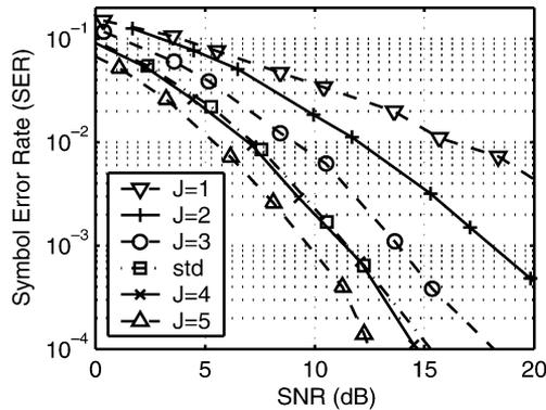
Fig. 2. SER as function of SNR for the proposed scheme with  $J = 2$  to five nodes, for the single-transmission  $J = 1$ , and for the standard TR-STBC (std) with four transmitters.
