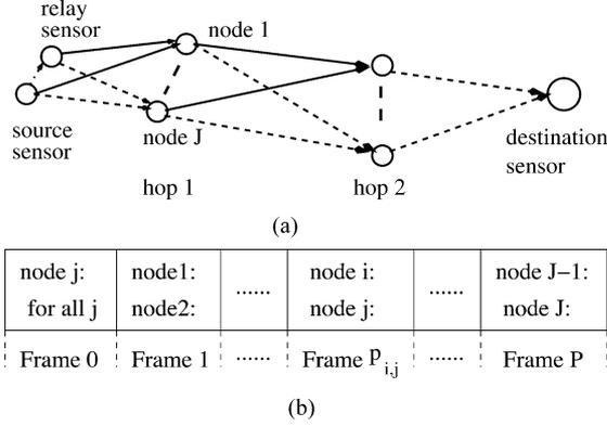
Fig. 1. (a) Multihop sensor network model with cooperative transmissions. (b) Space-time encoded transmission scheme, where a packet is subdivided into  $J$  blocks and is cooperatively transmitted by  $J$  nodes during  $P + 1$  time frames.
