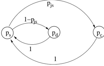
Fig. 2. Markov model for cognitive radio transmission under various jamming probabilities.
