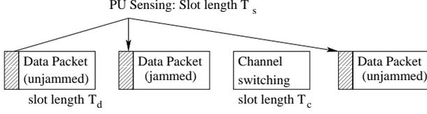
Fig. 1. Illustration of cognitive radio transmissions.
