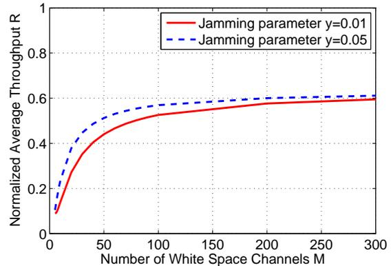
**Fig. 4.** Average throughput as function of number of white space channels, under various jamming conditions.
