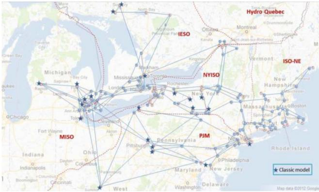
Fig. 4. Map of the NPPC 48-machine 140-bus system [29].
