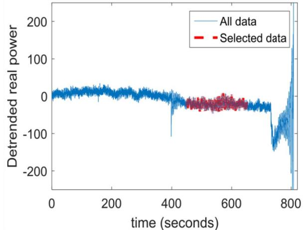
Fig. 12. Detrended real power on a major transmission line in the WECC system right before the power outage on 08/10/1996.
