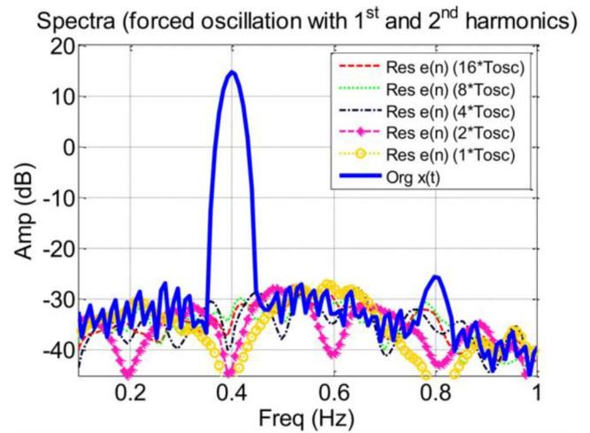
Fig. 8. PSDs of the original signal and the forecasting residuals in the **forced** oscillation case with 1<sup>st</sup> and 2<sup>nd</sup> order harmonics.
