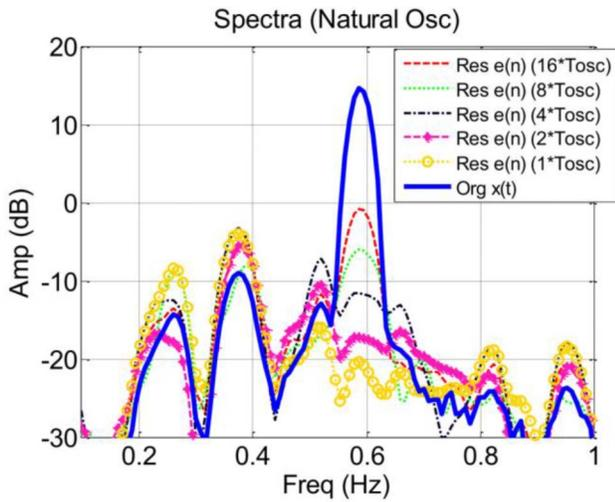
Fig. 6. PSDs of the original signal and the forecasting residuals in the **natural** oscillation case. (Here, “Res  $e(n)$  (16\*Tosc)” means the residuals from the forecast model whose lead time is 16 times of oscillation periods; “Org  $x(t)$ ” means the original data).
