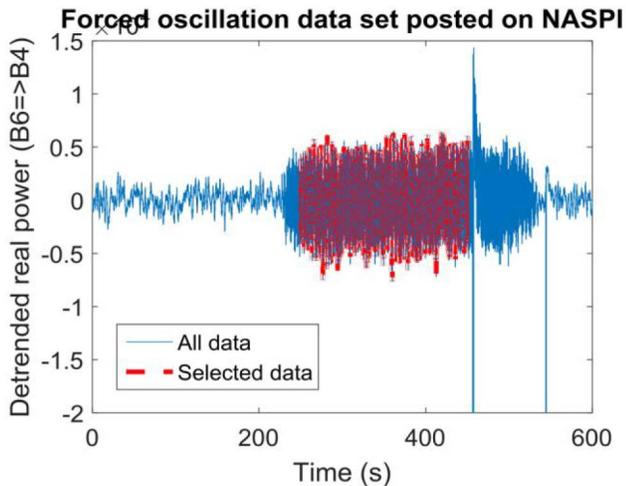
Fig. 14. Detrended real power from bus6 to bus4 during a sustained forced oscillation event posted on the NASPI website.
