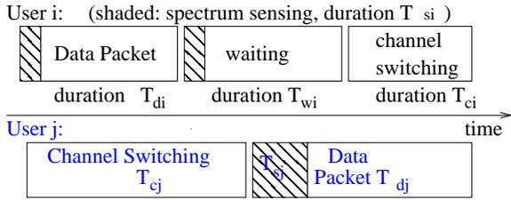
Fig. 2. Illustration of the cognitive radio operation with four basic states: spectrum/channel sensing, data packet transmission, waiting (idling) and channel switching.
