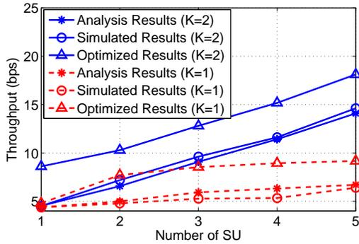
Fig. 4. CRN throughput when  $I = 1, \dots, 5$  SUs compete for  $K = 1$  channel or  $K = 2$  channels.
