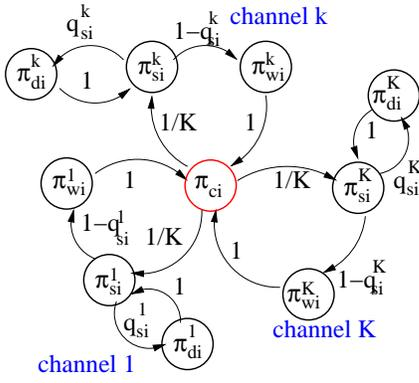
Fig. 3. Markov Model Bank (MMB) for heterogenous CRN. Only the Markov model for the SU  $i$  is shown. All other SUs have similar Markov models.
