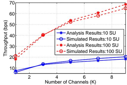
Fig. 5. CRN throughput as function of the number of channels, under two situations:  $I = 10$  SUs or  $I = 100$  SUs.
