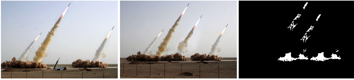
Figure 2.14: A typical copy-move manipulation, applied to a press photograph of an Iranian missile test. A non-functioning missile in the presumably original image (shown on the left, source: online service of the Iranian Daily Jamejam Today) was replaced by a copy of another missile (middle, source: Iranian Revolutionary Guards). The manipulated image appeared on the title page of a number of major Western newspapers [183]. The right image shows the output of Popescu and Faird’s [195] copy-move detector and marks near-duplicate regions.
