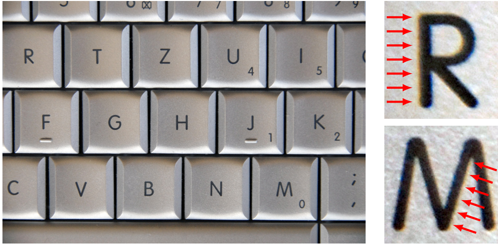
Figure 2.10: Lateral chromatic aberration in a digital camera image in the form of reddish color fringes along edges, which are marked by red arrows in the magnified (and contrast-enhanced) details on the right. The occurrence and strength of such color fringes in general varies with the position of the respective edge in the image (here, they only occur at edges facing away from the image center). The original image of an Apple MacBook Pro keyboard was acquired with a Nikon 18–200 mm zoom lens at a focal length of 150 mm.
