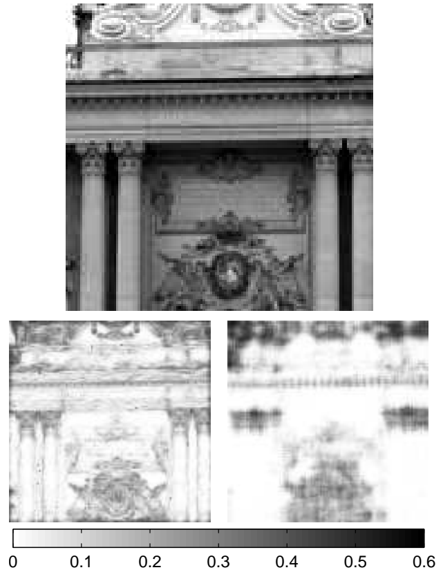
Fig. 5. Embedding probability for payload 0.4 bpp using HUGO (bottom left) and WOW (bottom right) for a 128 \times 128 grayscale cover image (top).
