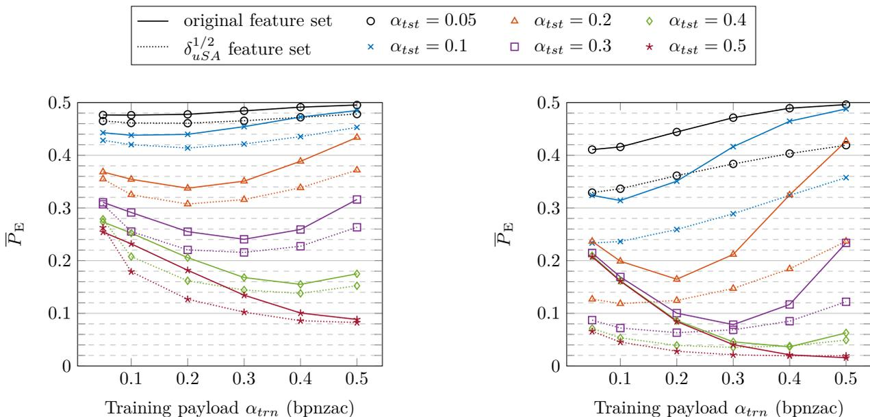
Figure 4. Detection error  $\bar{P}_E$  when training the detector on stego images embedded with payload  $\alpha_{trn}$  and testing on  $\alpha_{tst}$ . One testing payload corresponds to one curve. Left: J-UNIWARD with DCTR and  $\delta_{uSA}^{1/2}$ -DCTR, Right: UED-JC with GFR and  $\delta_{uSA}^{1/2}$ -GFR, both for JPEG quality factor 75.
