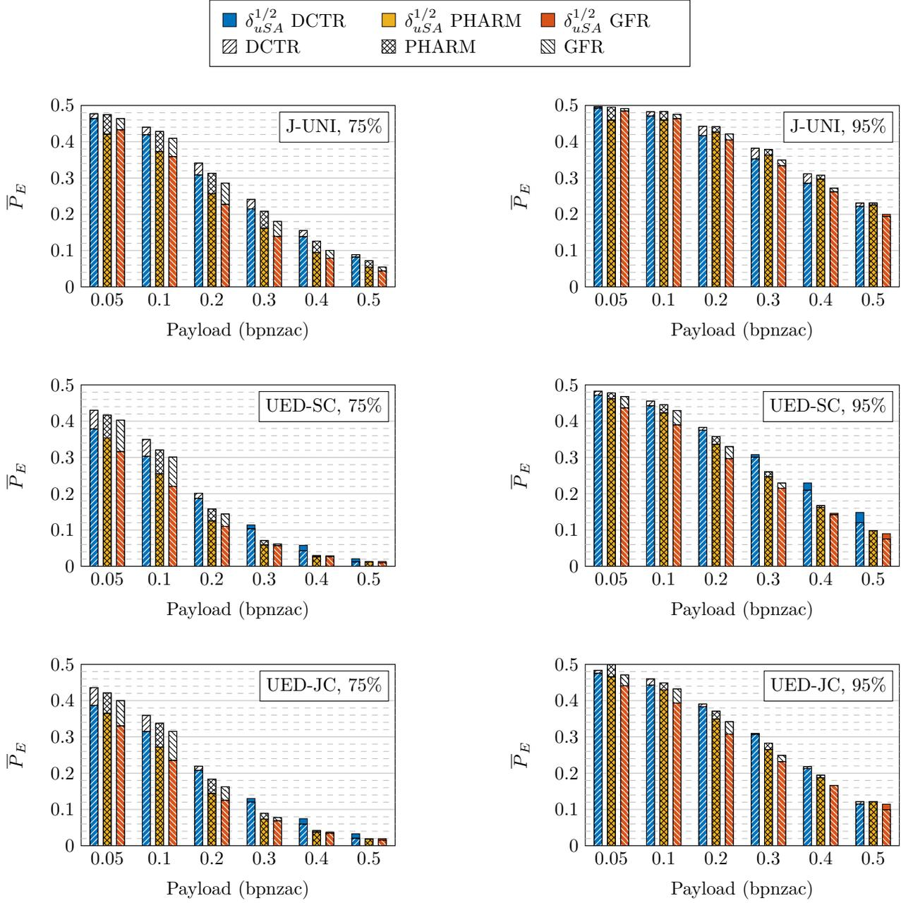
Figure 3. Detection error  $\bar{P}_E$  for three steganographic algorithms for DCTR, GFR, and PHARM features (patterns) and their selection-aware  $\delta_{uSA}^{1/2}$  version (solid fill) versus payload, JPEG quality factors 75 and 95.
