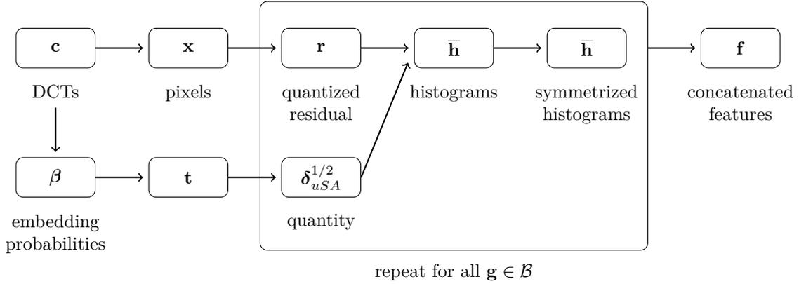
Figure 2. Diagram describing the proposed algorithm for the extracting of the  $\delta_{uSA}^{1/2}$  features.
