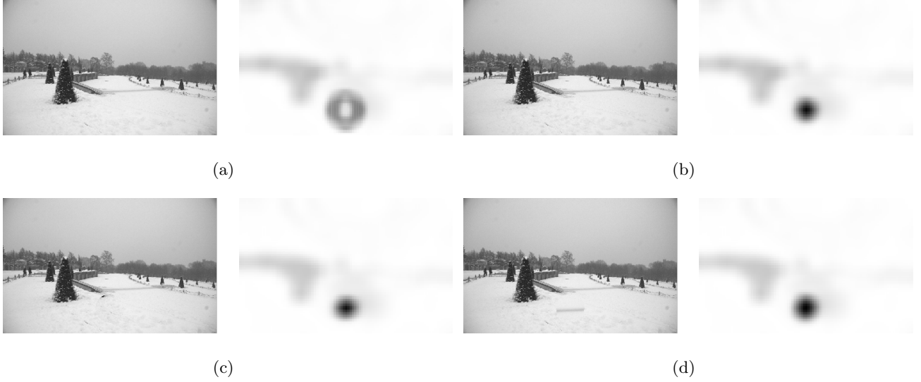
Figure 5. Detection output of Algorithm 1 applied to four types of area processing. The forged image (left), the output mask (right) for a) copy-paste forgery shifted by an odd number of pixels, b) rotation by 12 degrees, c) downsampling, d) upsampling.
