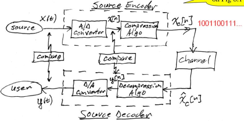
In practice this is how things get implemented. The A/D not only samples x(t) in time but it also discretizes the values – however, the discretization is very <u>fine</u>. The Comp. Algo. often includes further, coarser discretization
