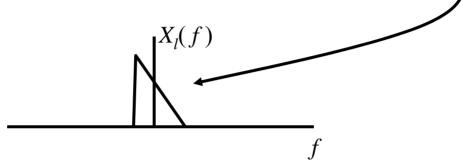
Note that because  $|x_i(f)|$  does not necessarily have even symmetry, the equivalent lowpass signal is complex valued,
