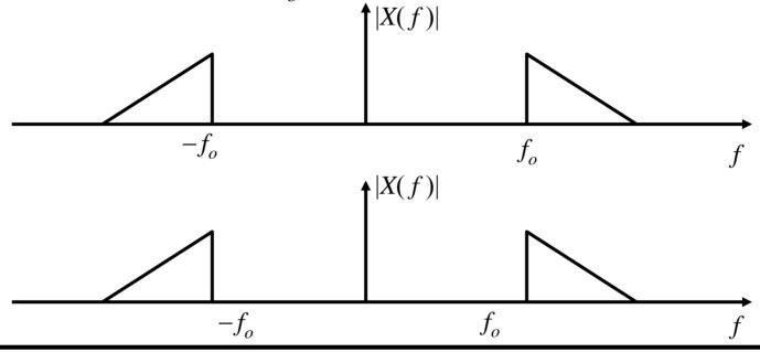
Bandpass signals are encountered when receiving radio frequency (RF) signals such as communication and radar signals.
