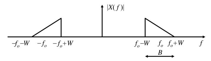
The **bandwidth** B of the bandpass signal = the width of the positive-frequency interval on which the signal is nonzero.
