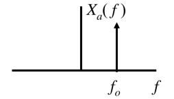
Then to get the **phasor**, we frequency-shift the analytic signal down by  $f_o$  to get:
