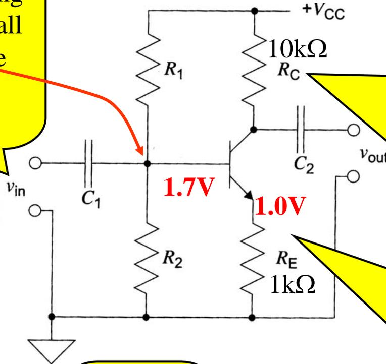
3. The collector current wiggles about the same amount:  $\Delta I_C \approx \Delta I_E$ . Causes the collector voltage to wiggle around 10V... But  $V_C$  goes down when  $V_B$  goes up (inversion!!!)
