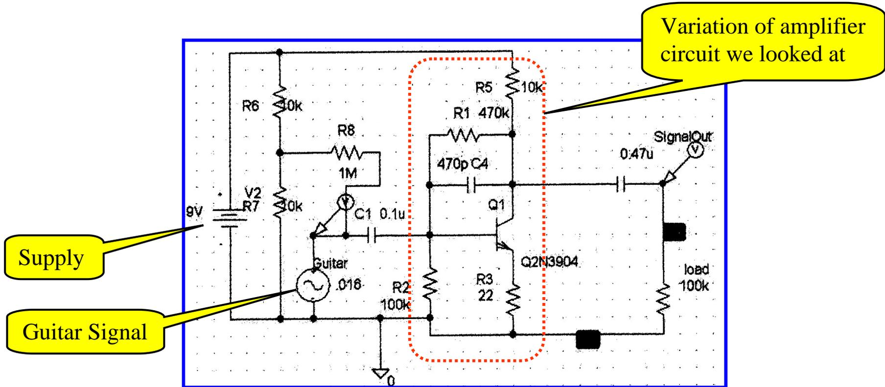
Partial Circuit for the Boss DS-1 Distortion Box for Guitar
