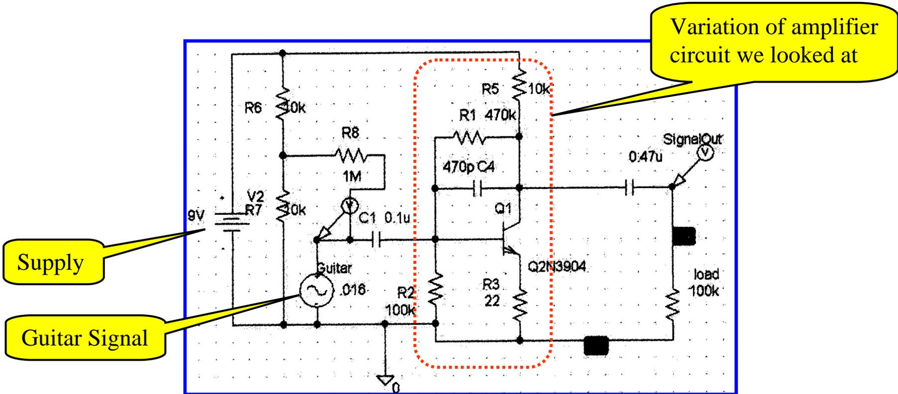
Partial Circuit for the Boss DS-1 Distortion Box for Guitar
