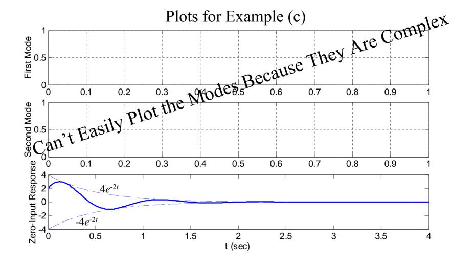
Because the characteristic roots are <u>complex</u>... have oscillations! Because real part of root is negative... \_\_\_\_\_!!!
