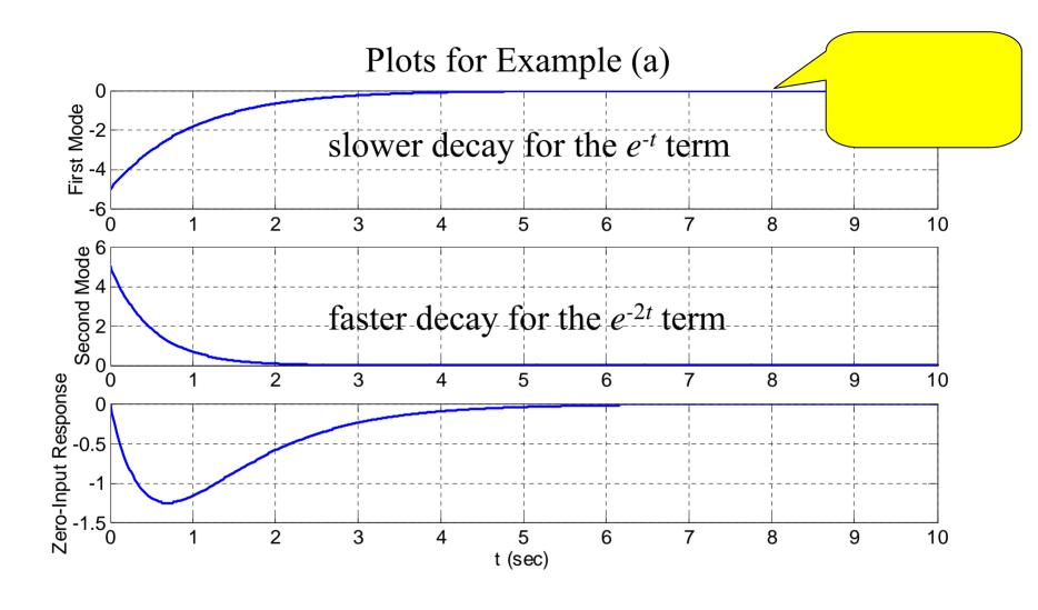
Because the characteristic roots are <u>real and negative</u>... the modes and the Z-I response all <u>decay to zero w/o oscillations</u>
