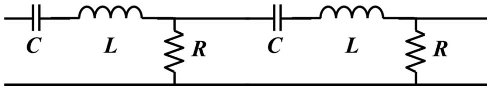
Our “cascade theory” only holds when attaching the 2<sup>nd</sup> system does not change how the first one behaves!
