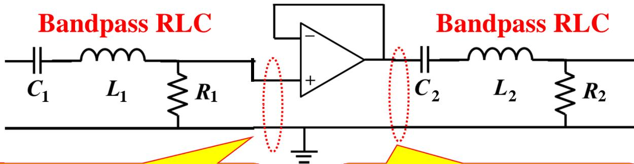
**VERY large input resistance of op amp prevents “loading” of first stage!**
