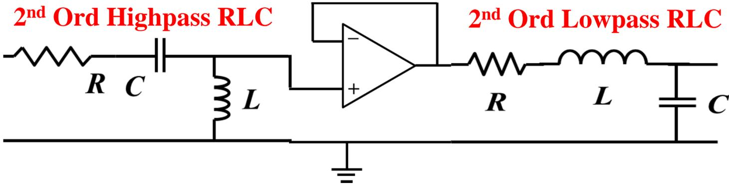
Although these ideas lead to workable circuits they are not necessarily the best... For one thing... they need inductors (which are big and can't be made in an IC!) There are other forms... See this link for the form used below.
