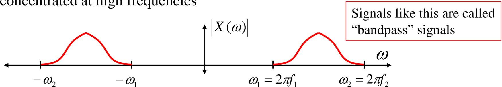
If the signal’s FT has negligible content for  $|\omega| \notin [\omega_1, \omega_2]$  then we say the signals BW =  $f_2 - f_1$  in Hz
