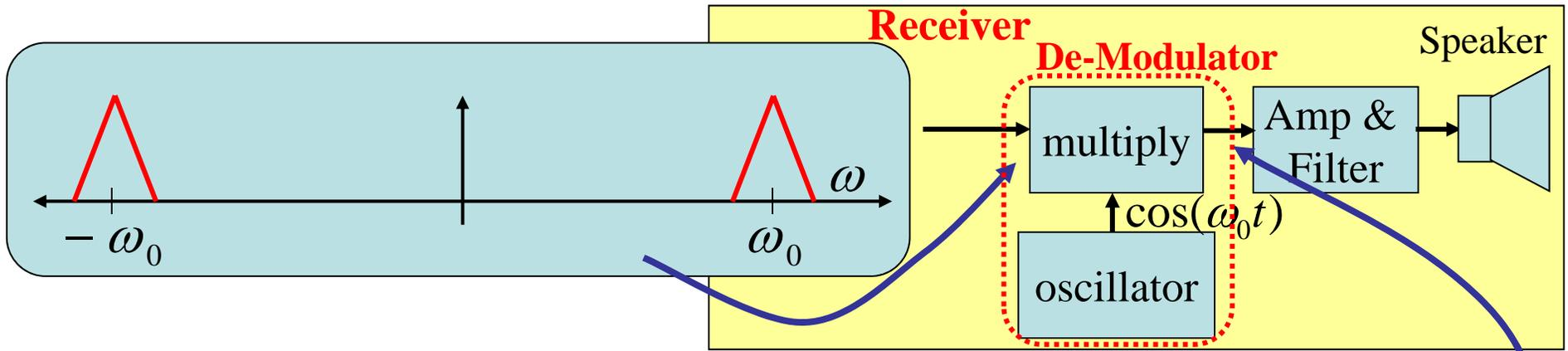
By the Real-Sinusoid Modulation Property... the De-Modulator shifts up & down:
