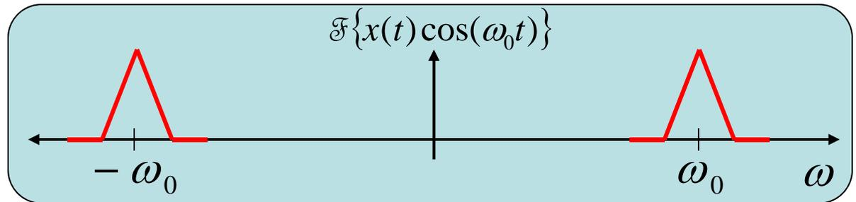
Choose  $f_0 > 10$  kHz to enable efficient radiation (with  $\omega_0 = 2\pi f_0$ )
