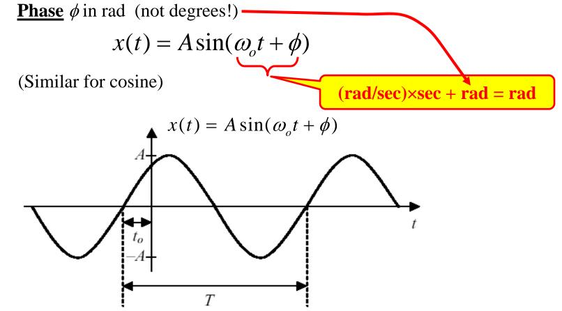
*T* is the Period of the sinusoid... it is related to the frequency  $\omega_o$  $t_o$  is a time shift... it is related the phase  $\phi$
