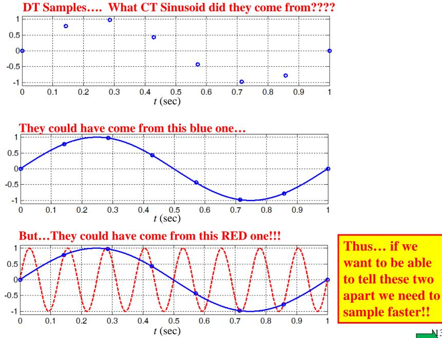
Let  $T_s$  be the time spacing between samples... Then  $F_s = 1/T_s$  as the "sampling frequency" in samples/sec.
