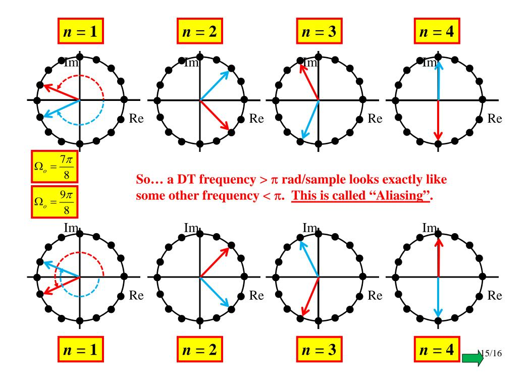
So to avoid this "aliasing" when sampling a CT sinusoid to make a DT sinusoid we must require that:
