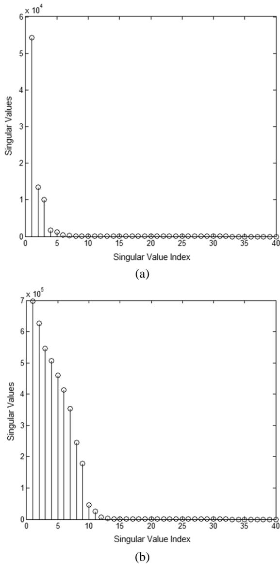
Fig. 1. Singular Values of CAF for two cases: (a) Noiseless signal, (b) Noisy signal
