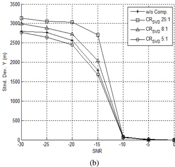
Fig. 3. Simulation results showing standard deviation for X and Y when we compress CAF using SVD-based compression. The four curves compare the cases (i) without compression, (ii) SVD-based compression with compression ratio of 25:1, (iii) SVD-based compression with compression ratio of 8:1, and (iv) SVD-based compression with compression ratio of 5:1.
