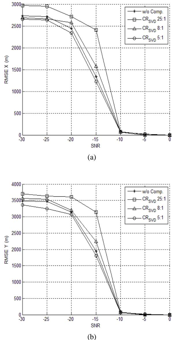
Fig. 2. Simulation results showing RMS error for X and Y when we compress CAF using SVD-based compression. The four curves compare the cases (i) without compression, (ii) SVD-based compression with compression ratio of 25:1, (iii) SVD-based compression with compression ratio of 8:1, and (iv) SVD-based compression with compression ratio of 5:1.
