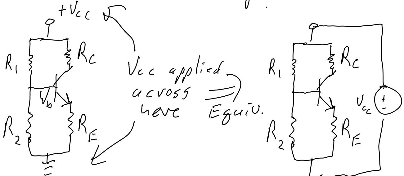
The goal of this biasing ② is to ensure that  $V_b$  is somewhere around  $\underline{V_{CC}}$  so that if we somehow make  $V_b$  wiggle up & down... there is room to wiggle:
