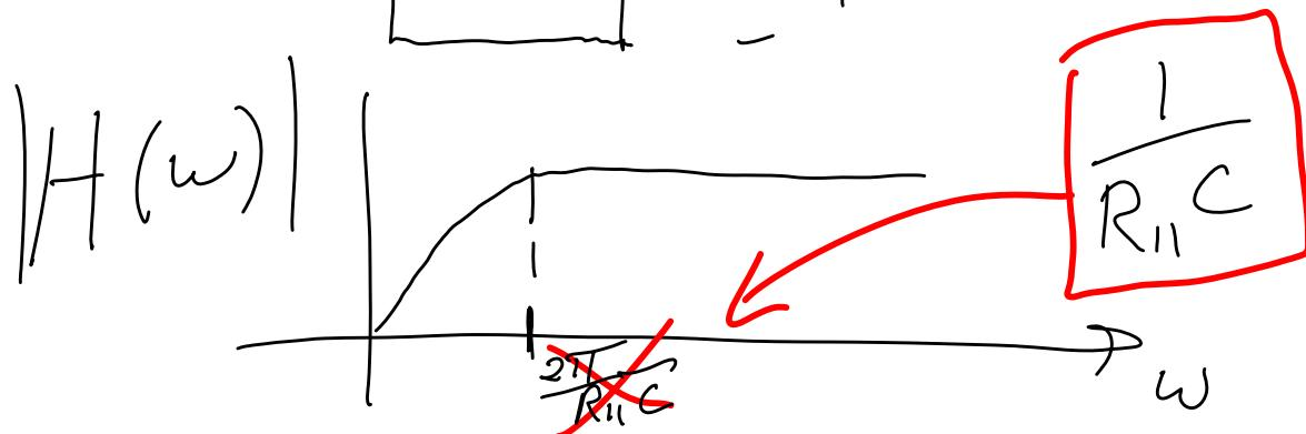
$$\Rightarrow V_{B_1}(t) = \sin(\omega_0 t) \quad \text{if } \frac{1}{R_{II} C} < \omega_0$$
