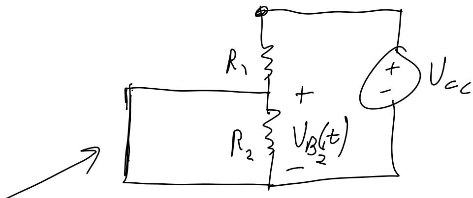
This short across  $R_2$  causes  $V_{B_2}(t) = 0$  !!
