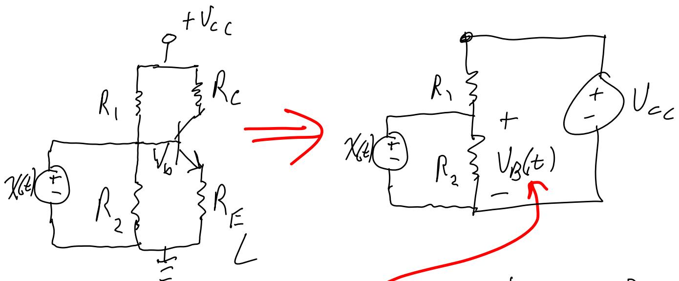
Does  $V_B(t) = \frac{V_{CC}}{2} + \sin(\omega t)$ ?
