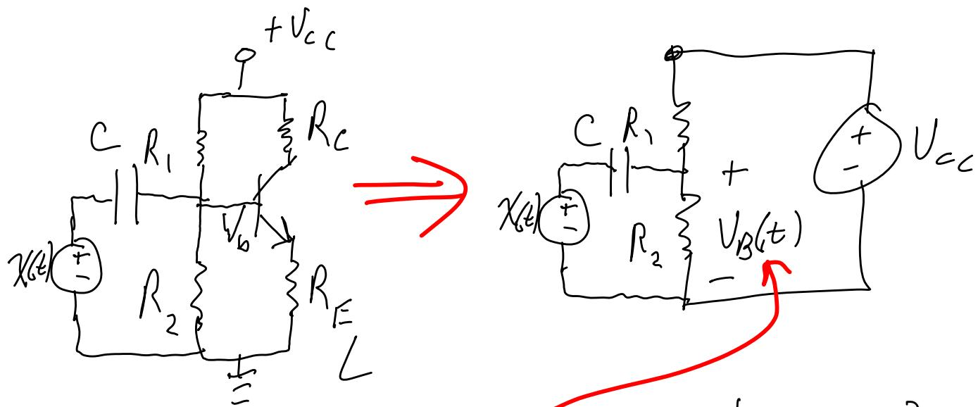
$$\text{Does } V_B(t) = \frac{V_{CC}}{2} + \sin(\omega t) ?$$
