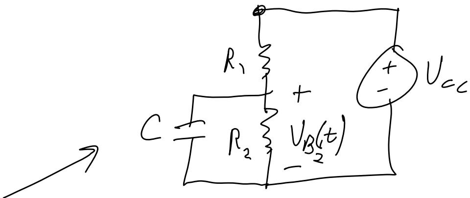
This cap. across  $R_2$  causes open circuit to act like DC source  $V_{CC}$ :
