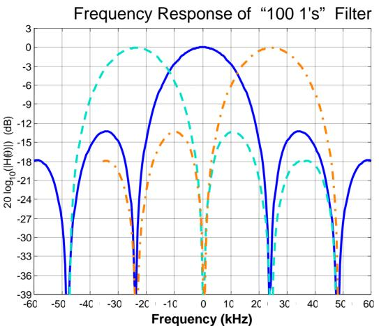
From this we see that in the middle of the doppler band we have very little impact from the aliasing, but at the edges of the doppler band there can be some severe aliasing. **Can we live with that?**
