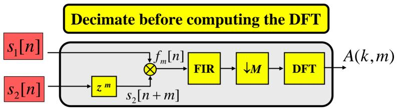
New # Samples after Decimating by 100: N = 240,000/100 = 2400 $\rightarrow$  New # Samples = 2400  $\rightarrow$  FFT size =  $2^{12} = 4096$
