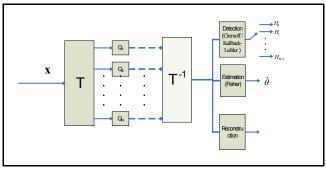
Figure 1: Scenario considered for study of data compression for multiple inference tasks
