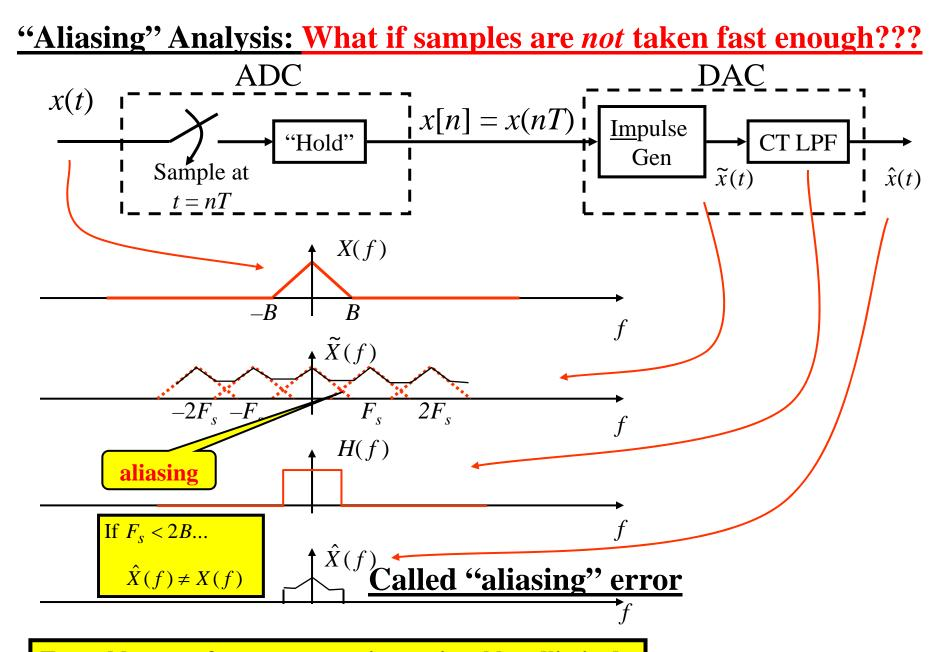
To enable error-free reconstruction, a signal bandlimited to B Hz <u>must</u> be sampled faster than 2B samples/sec
