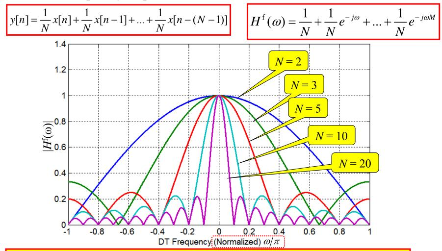
Increasing the length causes the passband to get narrower... but the quality of the filter doesn't get better... so we generally need other types of filters.
